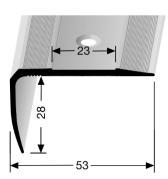
**Description:** Stair nosing "Reno" for slip-resistant insert, made of
